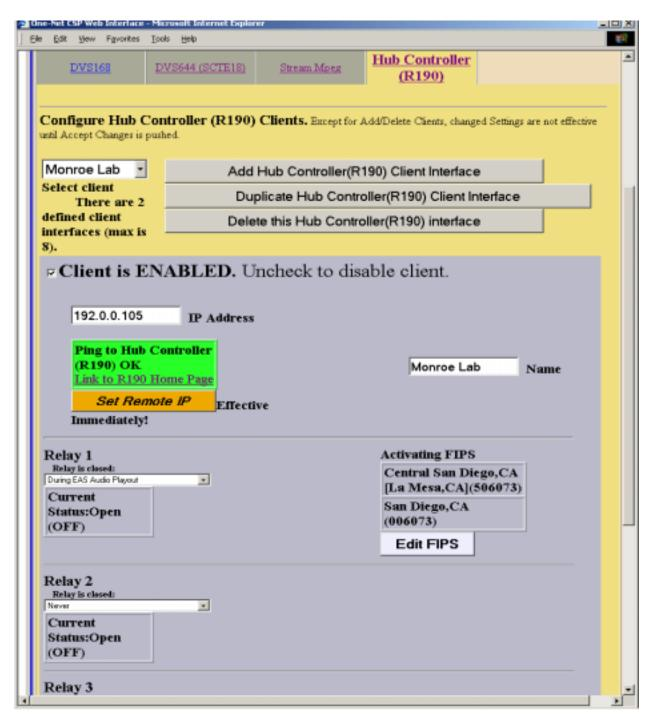
Note: Before enabling the Hub Controller, THE R190 MUST BE SET TO AN ADDRESS THAT IS WITHIN YOUR INTERNAL LAN. Follow the procedure included with the Hub Controller R190 for details.
