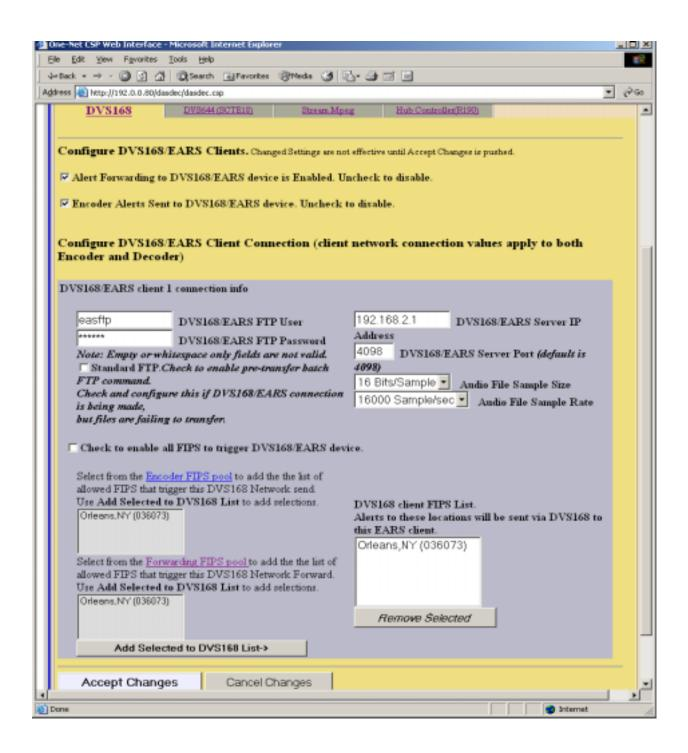
When an alert is forwarded to a DVS-168 client, a WAV file of the EAS audio is constructed and a text file of the alert details is constructed. These are FTPed to the DVS-168 client. Then a socket is temporarily opened from the One-Net to the DVS-168 client, and a control message is sent that describes the alert. The Operation Log will log each of these actions and their success or failure.
