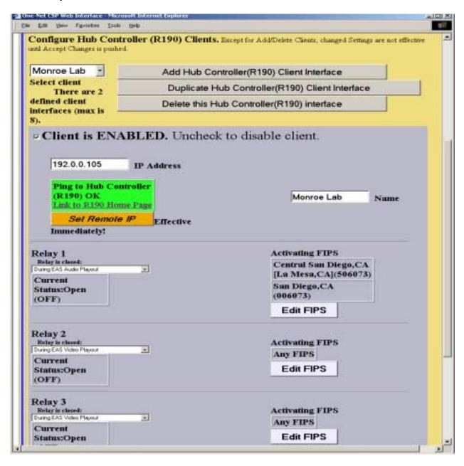
Relay activation can be programmed so that they only close when Alerts for specific FIPS areas are present. Click on the "Edit FIPS" button to select FIPS codes from the FIPS pools. When the desired FIPS codes are selected click the "Add FIPS selected above to the list" and they will be added to the FIPS list to the right. When finished, click on the "FIPS Editing Finished" button. Repeat this step for all of the required relays.
