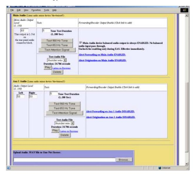
**NOTE:** The interface pages for Decoder and Encoder Audio display and reference audio output levels for certain features. These references always provide an active hyperlink into this page to allow for changes to audio output levels.
