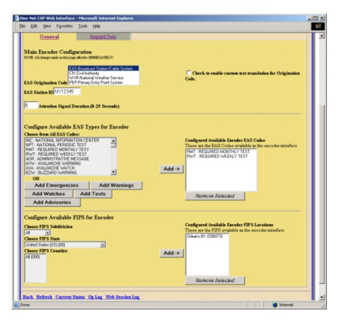
• To build or edit the list, choose an EAS code type from the pop down menu and click Add. Codes selected for encoding will appear in the Configured Available Encoder EAS Codes box to the right. Be sure and add all common EAS types that will be used when encoding alerts from this One-Net. If you find you are missing a code during encoding, you can edit the pool list at any time. To add a group of messages of a certain type, you can click one of the buttons (ie Add Watches).
