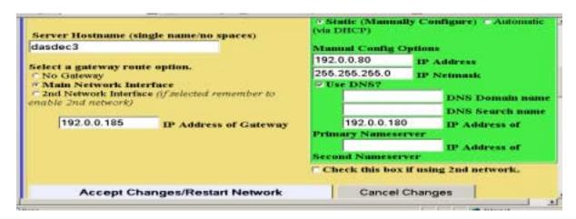
Enter the corresponding values. The example shows a new IP address of 192.0.0.80 and a netmask of 255.255.255.0, as well as a DNS and gateway configuration. To set the new values, select <u>Accept Changes</u>.
