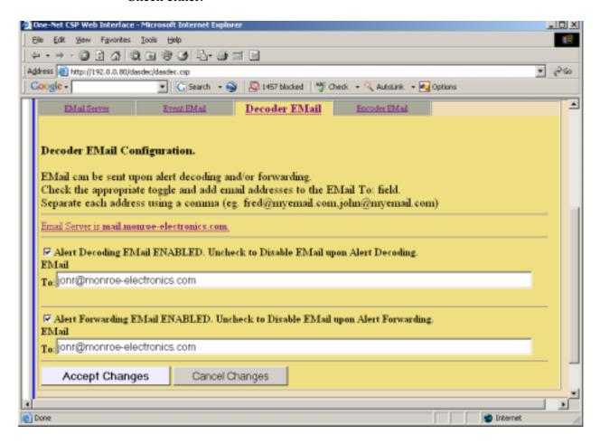
**Email upon Alert Decoding:** Check the box to disable or enable Email on Alert Decoding. If enabled, enter the Email address in the **Email To:** field.
