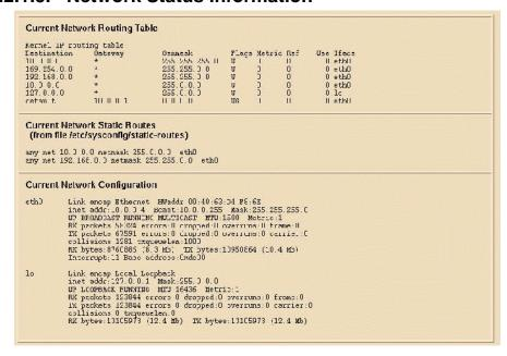
Tables at the bottom of the **Setup Network** page show the current network routes and network address information.
