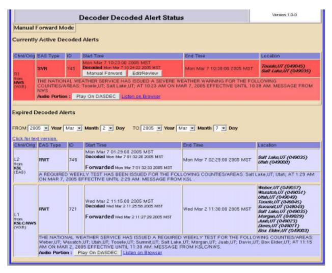
As can be seen from the example screenshot, every standard detail about the alert is presented in an easy to read table. In addition, the time the alert was decoded is displayed, as well as the time the alert was forwarded, if it was forwarded. Forwarded alerts are displayed on the **Forwarded Event Status** screen. See section 6.2.
