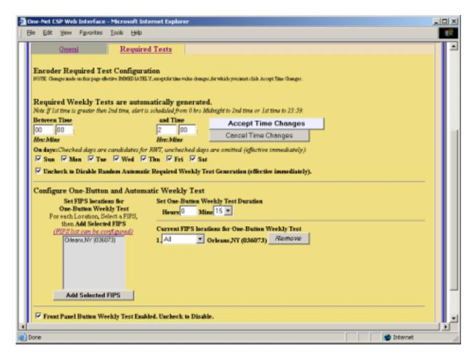
The **Required Tests** sub-page is used to issue pre-configured Weekly Test alerts. The One-Net can be configured to send a Required Weekly test with a single button push.
